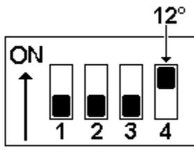
for a 8 cylinder engine fed with C.N.G. with 12° of spark advance
