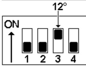
for a 4 cylinder engine fed with C.N.G. with 12° of spark advance
