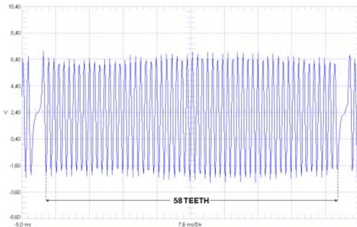
Measurement with engine at approx. 1.000 rpm
