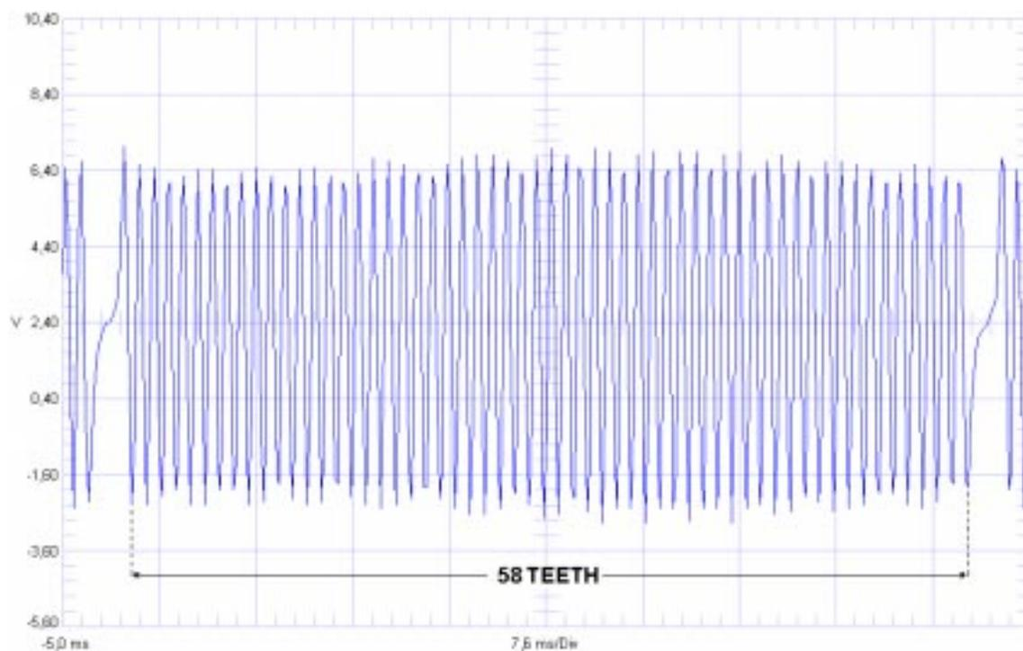
Measurement with engine at approx. 1.000 rpm
